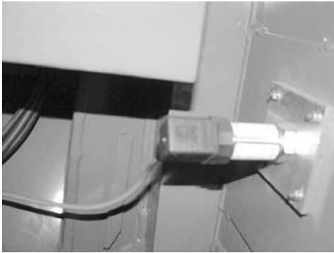
(b) Pressure sensor on skin of carbody
